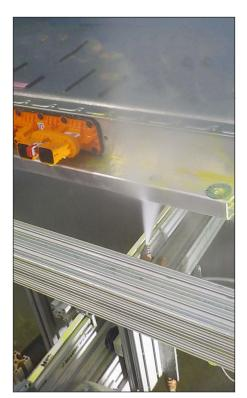
test conditions are executed and meet all the criteria associated with the first IP code numeral. There may be enclosures that do not meet both the protection against foreign objects and protection against access for a first IP code numeral. ISO 20653 and IEC 60529 provide the opportunity to classify an enclosure's protection against access with an "additional letter". The "additional letter" will indicate the test that is to be conducted to verify compliance.
